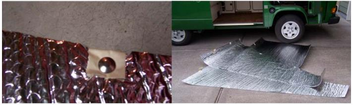
Be sure to mark which side/front for snap installation. Using a simple hammer-in snap kit, install snaps onto the Reflectix side panel tops. For the front-facing sections of the side panels, use the snaps to attach Velcro strips (soft fuzzy strip). Make them 6" long. Carefully plan this so it will lay proper to catch the receiver Velcro on the front panel later. I used (2) female snaps on the tops, and (2) (any gender) snaps to hold the Velcro at the front. (See the photos)
