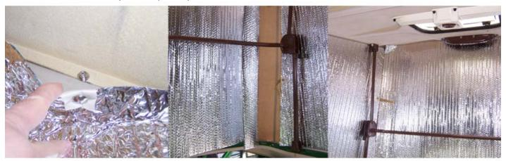
Pre-drill the hole for the male snaps on the pop top edge. Use Stainless screws in the male snap. Again, plan carefully as you only get (1) try. Use heavy duty outdoor-rated double sided 3M adhesive tape to secure the (bristle strip) Velcro to the Reflectix front panel. That is it. The finished panels install easily, and stow well in the back of the bunk area. Insulation holds heat in, allows ventilation in back. 2011 plummerdesign.com
