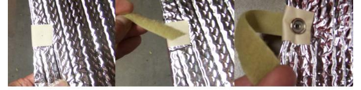
From a  $48'' \times 25'$  roll of Reflectix, cut three sections. The sides are 89'' long at the bottom  $\times 83''$  long at the top  $\times 10''$  tall at the back  $\times 43''$  tall at the front (this is an offset cut). The front panel section is  $50'' \times 43''$ . The back is open for ventilation and has no panel. Once cut, iron on some snap backer fabric using standard iron-on knee patch material. This will keep the Reflectix material from ripping, a good thing.
